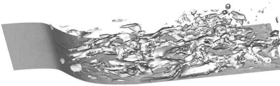
Fig. 21. Iso-surfaces of the streamwise vorticity obtained by DES of oscillatory suction/blowing flow control case.
